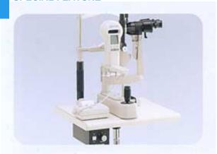
Sagittal radius measurement on the slit lamp arm. 4-LED fixation lamps at 25° angle against the keratometry axis.
